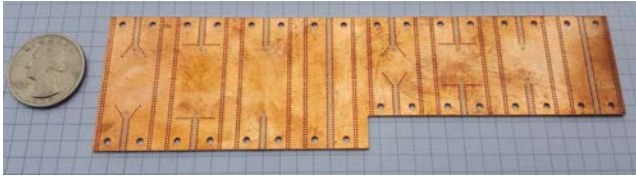
Fig. 7: Photo of all fabricated PCB structures next to a US quarter. Each square in the background has 5mm sides.
