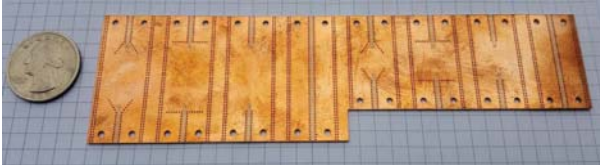
Fig. 12. Photo of all fabricated PCB structures next to a US quarter. Each square in the background has 5mm sides.
